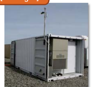
Mobile noble gas measurement system (TXL : Transportable Xenon Laboratory) 11
